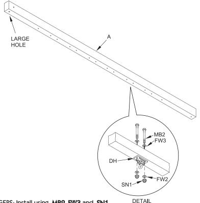
PART DH HANGERS: Install using  $\,$  MB2, FW3, and  $\,$  SN1 (See Detail)
