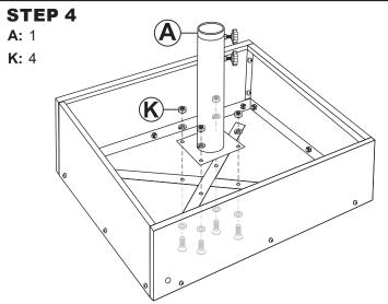
Secure Umbrella Pole (A) to the base using four M8x25mm Bolt Sets (K). **NOTE:** Use the flat washer next to the bolt head and the split washer next to the nut.
