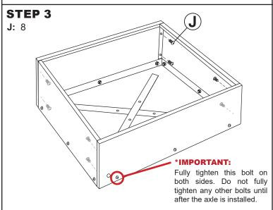
Loosely affix the side panels using two M6x15mm Bolts (J) in each corner.
