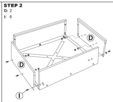
Align two Short Panels (D) with the base and loosely secure each panel using three M6x12mm Bolt Sets (I). **NOTE:** Use the flat washer next to the bolt head and the split washer next to the nut.
