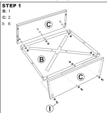
Align two Wheel Side Panels (C) with Base (B) and loosely secure each panel using three M6x12mm Bolt Sets (I). **NOTE:** Use the flat washer next to the bolt head and the split washer next to the nut.
