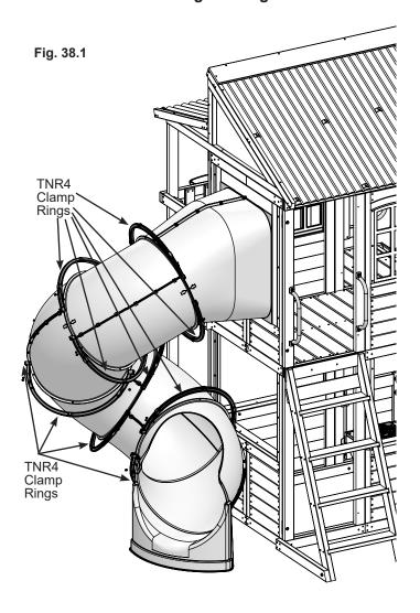
Note: For ease of assembly bottom set of clamp rings can be rotated 90 degrees to install bolts.
