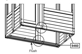
Note hole orientation in Fig. 3.7, 3 screws into large panel and 2 into the small panel.
