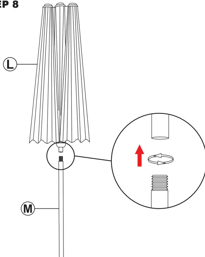
Twist Pole (M) clockwise into the bottom of Umbrella (L) until they are fully engaged.
