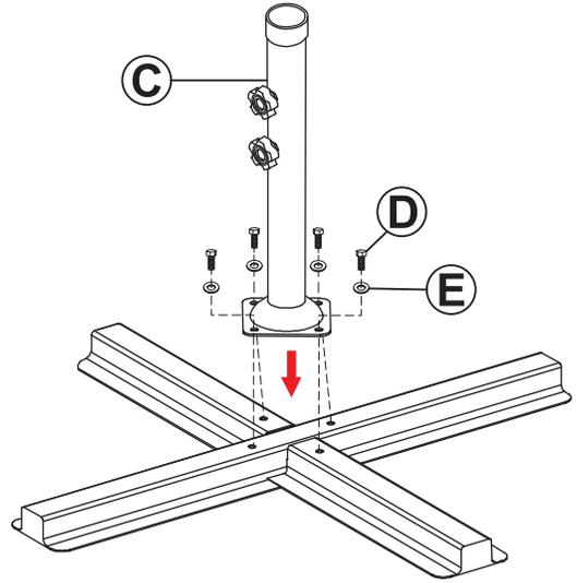
Securely fasten Pole Support (C) to the crossbars using four Washers (E) and Bolts (D), as shown.
