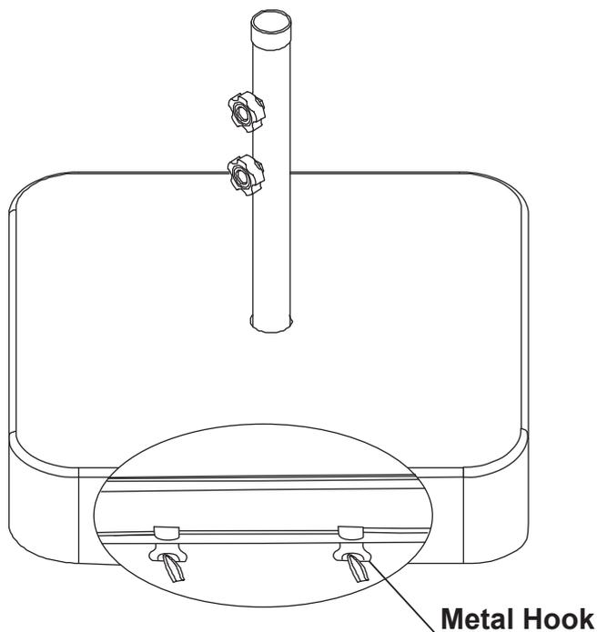
Locate the metal hooks on the base cover and secure them to the base frame, as shown.
