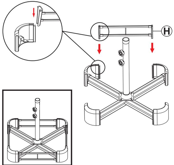
Slide four Base Frames (H) between the base corners, as shown.
