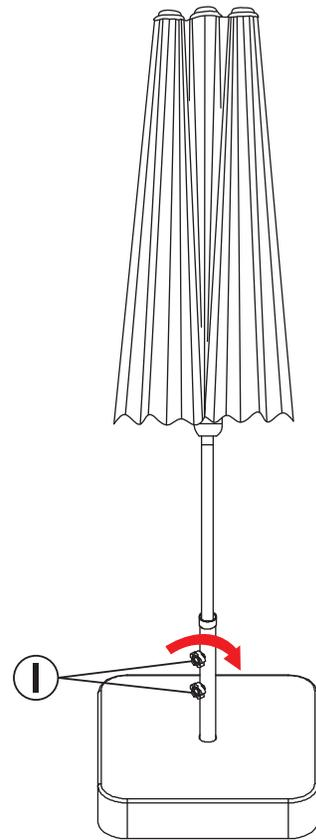
Tighten Threaded Knobs (I) to secure the umbrella.
