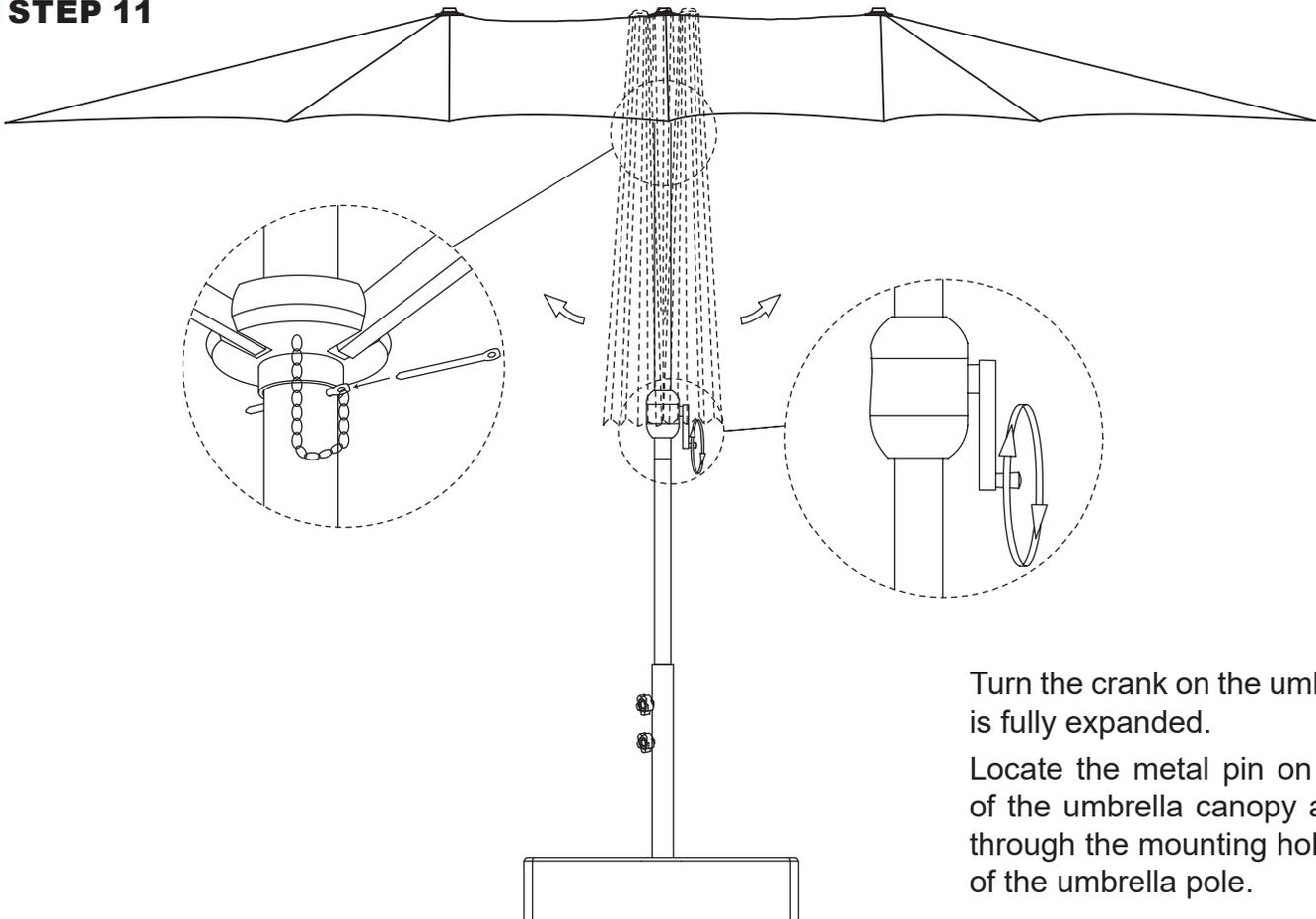
Turn the crank on the umbrella until it is fully expanded.
