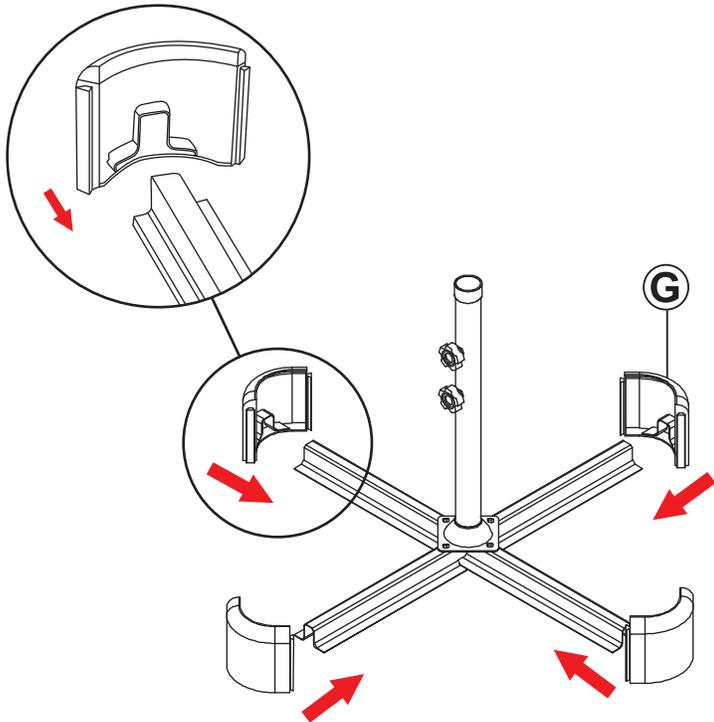
Attach four Base Corners (G) to the legs, as shown.
