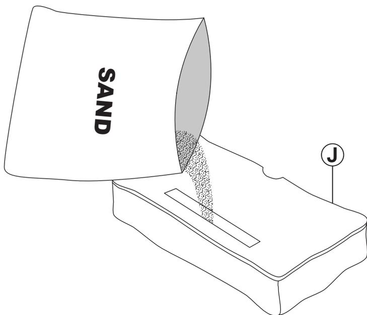
Fill two Sand Bags (J) with sand. Press the hook and loop fasteners together to close the bag.
