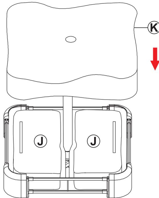
Place the sand bags inside the umbrella base and slide Base Cover (K) over the pole support, onto the base.
