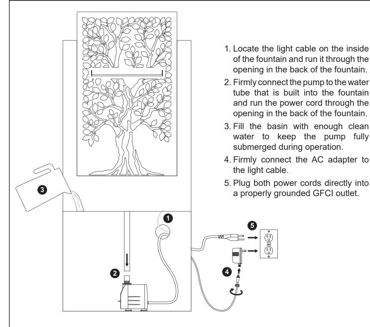
NOTE: When first used, there may be air trapped in the pump. It may take several minutes for trapped air to escape, allowing water to flow.
