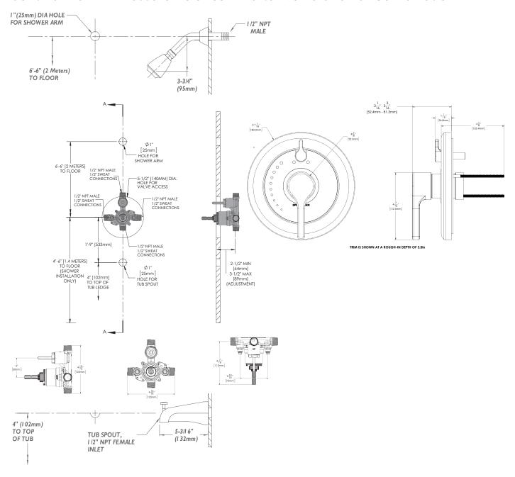
NOTE: 1. All dimensions are in inches (millimeters) unless otherwise specified and are subject to change without notice. 2. Unless otherwise specified, all inlets and outlets are 1/2" female copper sweat. 3. For ADA mounting locations, consult ADAAG, ANSI A117.1, or static regulations
