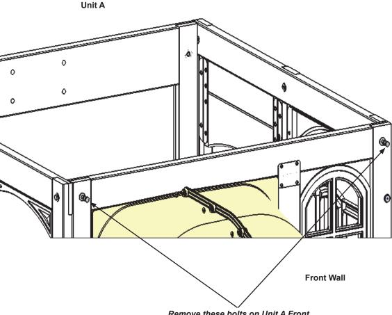
Remove these bolts on Unit A Front Wall, keeping lock washers and flat washers for next step. Do not remove the t-nuts.
