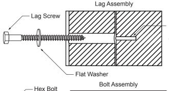
Before mounting Lag Screw, use factory drilled holes as guides to drill 1/8" pilot holes
