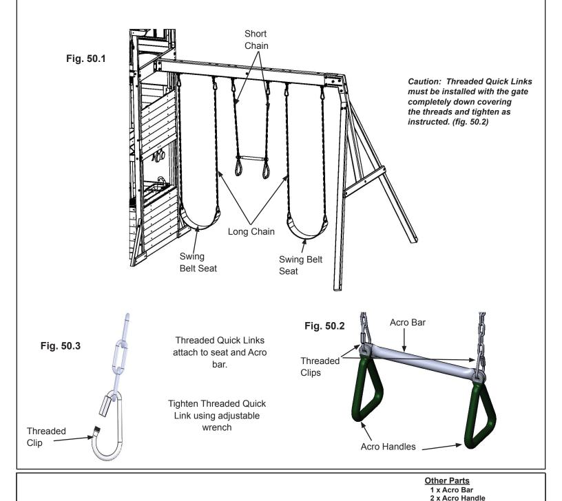
2 x Swing Belt Seat 2 x Short Chain 4 x Long Chain 6 x Threaded Quick Link
