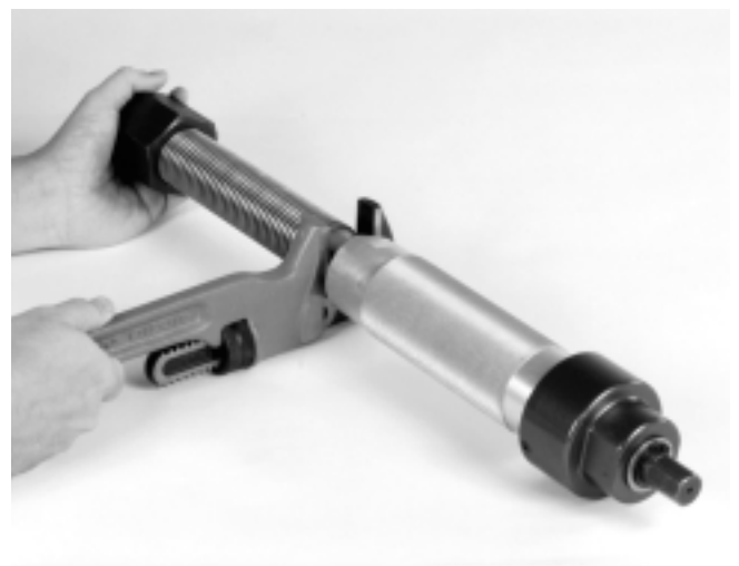
Figure 1 – Assembling Valve Adapter Onto Feed Screw
