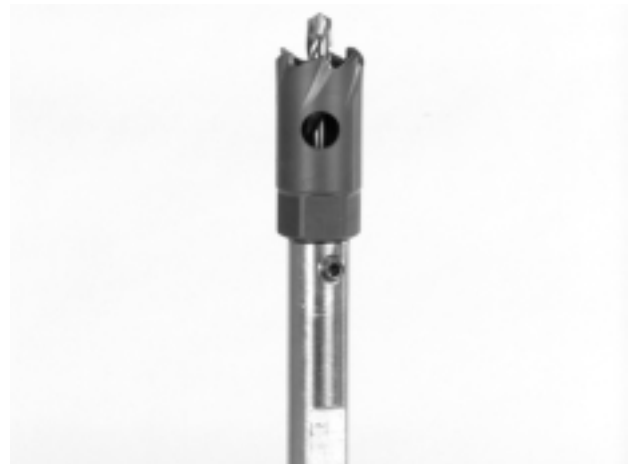
Figure 4 – Installation Of Pilot Drill
