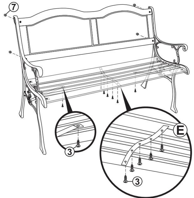
Secure the side braces to the seat using M3x15mm Screws (3).
