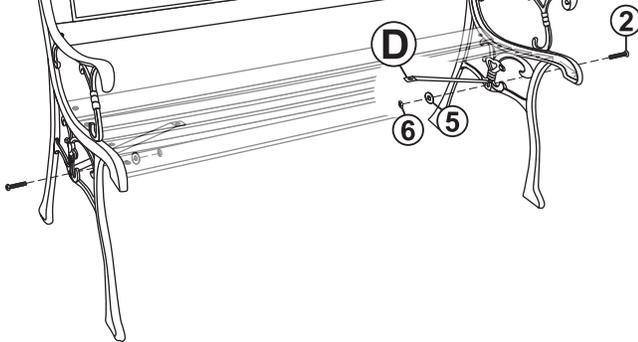
Attach Side Braces (D) to the arm panels using M6x20mm Bolts (2), Washers (5), and Nuts (6).
