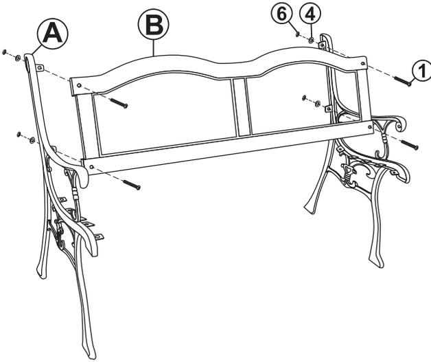
Fasten Backrest (B) to Arm Panels (A) using M6x30mm Bolts (1), Washers (4), and Nuts (6).
