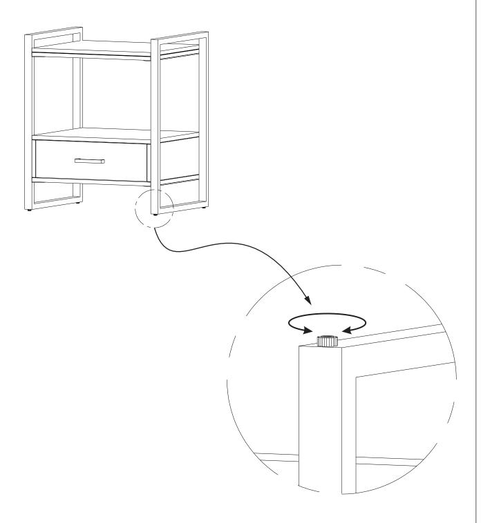
Note: Levelers on bottom of Sides can be adjusted if floor is unven.
