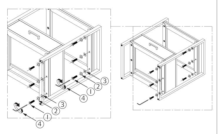
I. Repeat Steps 2 and 3 to attach the second Side B to Top A and Bottom C.
