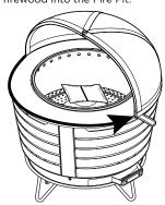
Use protective gear to grab the handle and close the Fire Pit Screen after lighting a fire as the screen will be hot.
