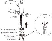
2.Adjust the position of the faucet and secure it with the fixing kit as photo.
