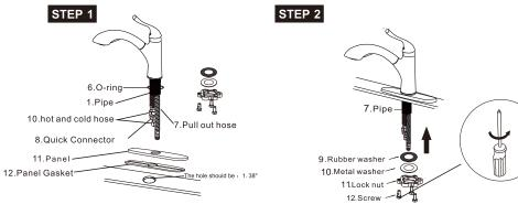
1.Position the faucet, deck plate and o-ring on the installation surface. And then put the faucet into center hole.
