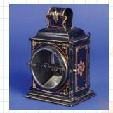
In 1872 Andrew Dick made an improvement to an existing locomotive signal light. The lamp would include a stationary and movable headlight so that train workers could identify the train name or number as it came into the station at night.
