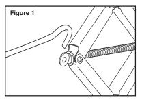
Unfold the speed handle and use one hand to hold the front part of the handle while using the other hand to slowly rotate the end of the handle clockwise to desired height. (See figure 2)
