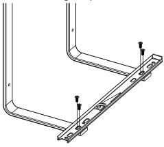
3) Once both inner slides member are attached to both sides you are now ready to attach the brackets to a underside of your shelf using the provided (4) wood screws.
