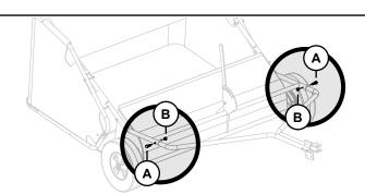
11. Align and attach the Left and Right-hand Mount Brackets (3 & 4) to inside edges of the Tow Tubes on Sweeper using previously removed hardware.
