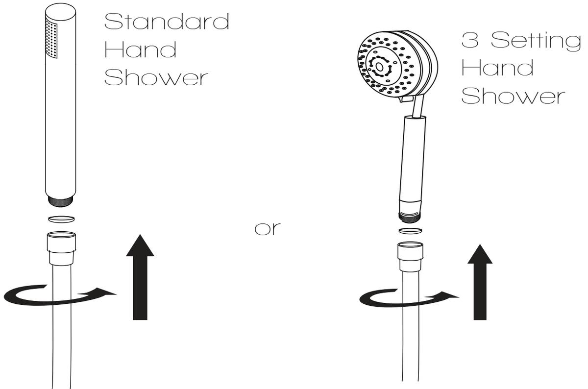
**Step 2A** Finally, install the shower wand to the hose, as shown.
