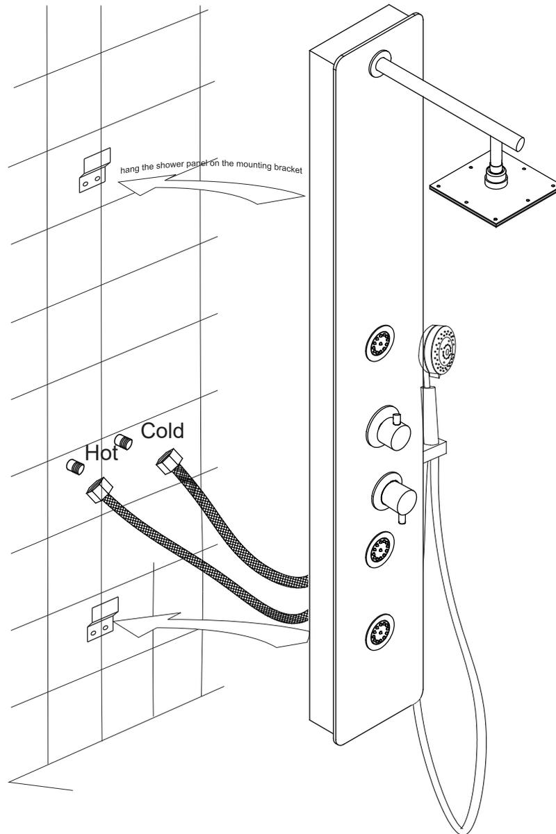
**Step 4A** Screw the cold and hot water hose from the shower panel to the supply lines in the wall.
