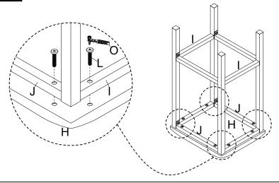
Stand stool up on an even surface and check that it is balanced. If there is a slight wobble, apply downward pressure in the corner where a leg is uneven. Keeping pressure in that corner, tighten all bolts. If balanced, apply downward pressure evenly in the center and tighten all bolts. Do not over-tighten beyond hole depth.
