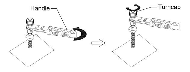
Attach Left Side Frame (B), Right Side Frame (D) and Middle Frame (C) to the Table Top (A), insert the Bolt (L), turn the Ratchet Tool (O) to tighten them.
