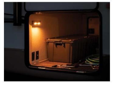
When the power switch is in the ON position, the motion detector will trigger the camper step light to illuminate when movement is detected in the surrounding area. It will turn on for 15 seconds before shutting off if no further activity is detected.
