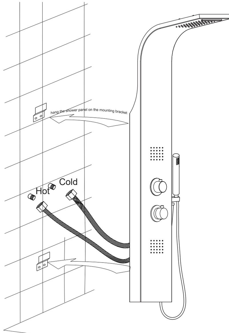
**Step 4A** Screw the cold and hot water hoses from the shower panel to the supply lines in the wall.
