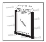
Cut head flashing so it will extend beyond jamb flashing. Finally, lay weather-resistant barrier over head flashing. Apply sheathing tape over both diagonal cuts.
