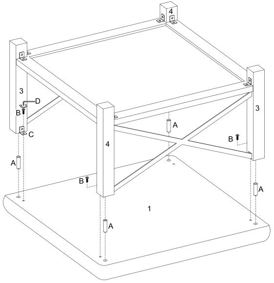
Insert wooden dowel (A) into part (1) ,using bolt (B) secure L type connector into parts (3,4) to part (1) with hex key (D) as per diagram.
