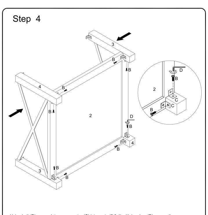
Using bolt (B) secure L type connector (C) into parts (2,3,4) with hex key (D) as per diagram.
