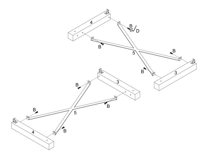
Using bolt (B) secure part (5) into parts (3,4) with hex key (D) as per diagram.
