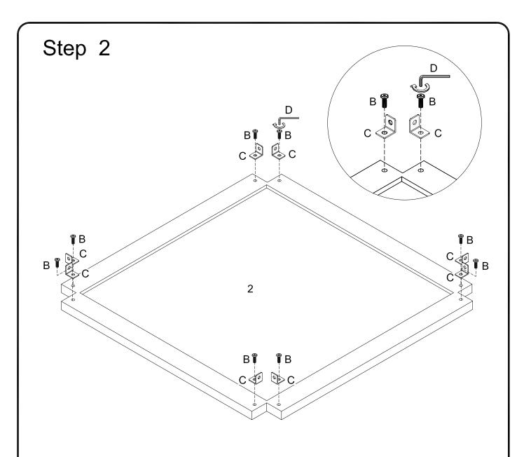
Using bolt (B) secure L type connector (C) into part (2) with hex key (D) as per diagram.
