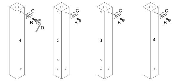
Using bolt (B) secure L type connector (C) into parts (3,4) with hex key (D) as per diagram.
