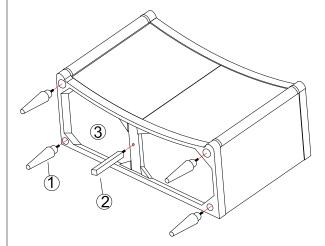
Install the acrylic legs (1) & center leg (2) in clockwise direction into the bottom of the case (3). Remove them by the reverse way.
