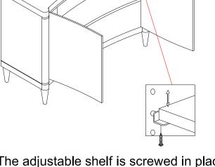
The adjustable shelf is screwed in place to avoid damage during transit.
