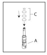
6. Using capsule (D) lubricate new o-rings (C).
