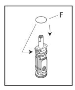
9. Using capsule (D) lubricate new side seals (G) and o-ring (F).
