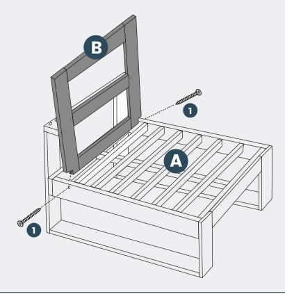
7 Attach Part B Backrest to Part F Back Support with 2 pcs of Hardware #1 Screw.
