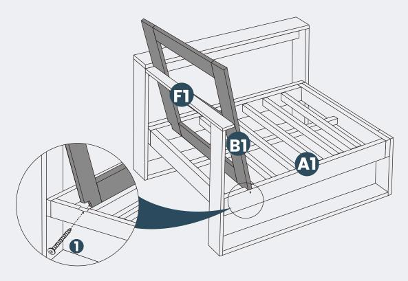
Attach Part B1 Backrest to Part G1 Chair Left Arm with 1 pc of Hardware #2 Screw.
