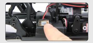
Check the operation of the throttle and steering. Pulling the throttle trigger back will drive the car forward, pushing the trigger forward once will apply the brakes while pushing the trigger forward twice will drive the car in reverse. Turning the wheel to the right will cause the car to turn right and vice versa.
