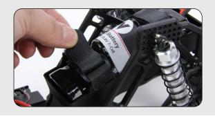
Ensure the radio switch is in the OFF position, then connect the battery to the ESC.
