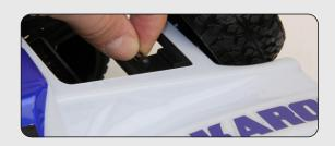
Locate the battery cradle at the back of the car, release the hook and loop tape and withdraw the battery pack.
