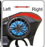
Use the throttle CH1 and steering trim Ch2 dials to fine-tune the controls of your car. In doing so, ensure that your Karoo Desert Truck tracks in a straight line. Also that it doesn't creep forwards or backwards at zero throttle.
