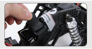
2 Locate the receiver box and, using a 2mm hex driver, remove the protective cover.
