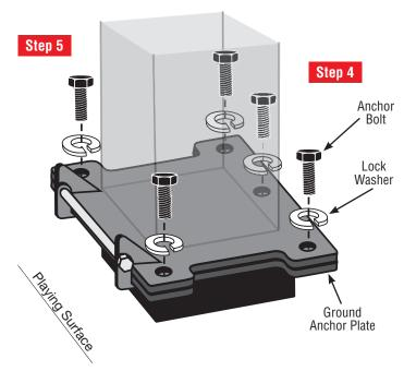
**Step 6:** Snug tighten the five anchor bolts, then check goal assembly with a level and inspect visually to determine if it is parallel and plumb to the playing surface.
