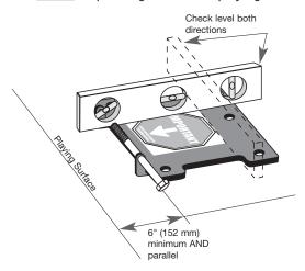
**Step 6:** Position 4" ground anchor (Item G2440) in center of hole with hinge side toward and parallel with playing surface. Using a level, ensure the anchor is level front-to-back and left-to-right. All edges of the ground anchor must be 6" (15.2 cm) away from all sides of hole and the top of the ground anchor within a range of 1"- 3" (25-75 mm) above the level of the playing surface.
