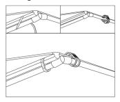
• Continue wrapping the assembled Misting Tube around the complete circumference of umbrella. Position a Tee with Nozzle at the end of each umbrella rib.
