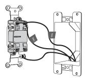
Carefully pull out outlet from wall. Label wires connected to existing outlet box and disconnect wires.
