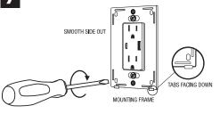
Place the mounting frame over your installed outlet and secure it using provided screws.
