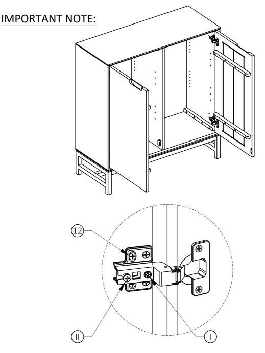
Tighten the Screw marked (1) to fasten hinge. The door may need to be adjusted so that all the spaces between the door and the unit sides are equal. To adjust, follow instructions:
