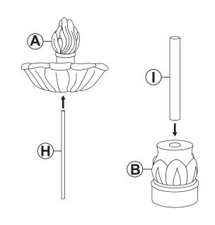
Install Water Tube (H) to the bottom of Topper (A). Install PVC Tube (I) into Top Column (B).
