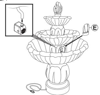
Firmly connect the water tube to the pump. Place Pump Access Cover (E) over the opening.
