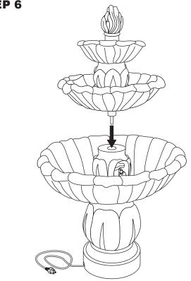
Install the assembled top tiers on the bottom column.
