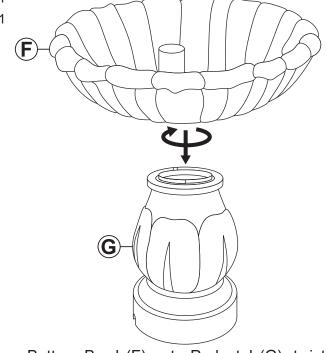
Place Bottom Bowl (F) onto Pedestal (G), twist to lock in place.
