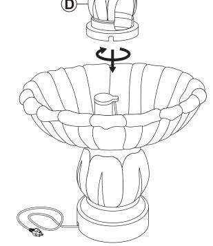
Install Bottom Column (D) onto the bottom bowl, twist to lock in place.
