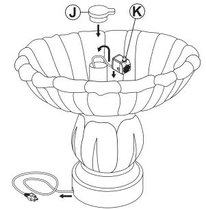
Place Pump (K) in the center of the bottom bowl and run the power cord through the tube that is built into the bottom bowl and under the groove in the bottom of the pedestal. Install Leak Guard (J) over the tube.
