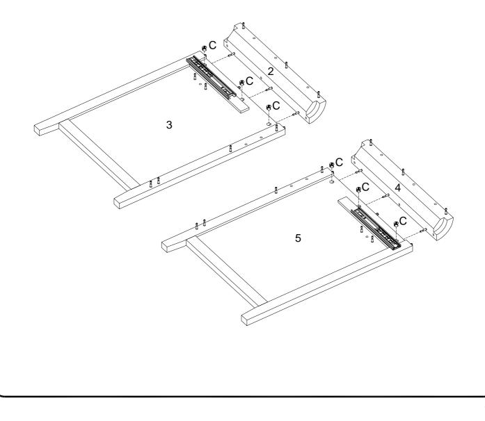
Attach the Left Side Panel (3) and Left Corner Panel (2) to the body of the Desk. It will attach to the Desktop Panel (1), Drawer Support Panel (9), Back Panel (6), and Support Panel (7). Secure with Cam Locks (C).
