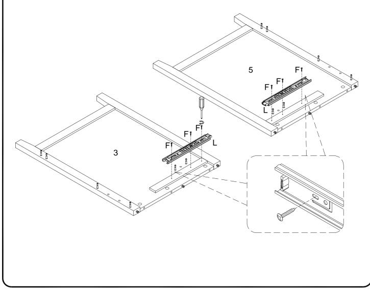
Next, you will attach a Drawer Glide (L) cabinet member on each side of the Drawer Divider (8). Ensure that you are matching to the correct sides according to the diagram.
