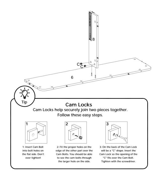
Now, you'll attach the Desktop Panel (1) to the Back Panel (6) and the Drawer Divider (8). Using Cam Locks (C), secure with a screwdriver.
