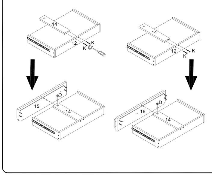
Flip the drawer over and secure Front Drawer Panels (15) and (16) to both Side Panels (10) and (11) using Cam Locks (D).
