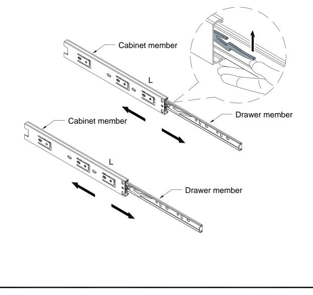
Attach one Drawer Glide (L) cabinet member to the Left Side Panel (3) and one to the Right Side panel (5) using 12mm Screws (F).
