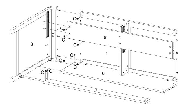
Repeat the same process with the Right Side Panel (5) and Right Corner Panel (4). Secure with Cam Locks (C).
