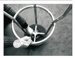
If the stool legs are uneven, insert a shim (supplied) between the foot pad and the stool leg to level the stool.
