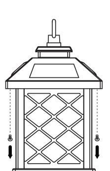
2 Replace the current lithium-ion battery with a new lithium-ion 18650 1500mAh to 3400mAh 3.7V. Reattach the lid.
