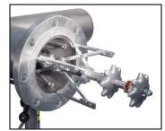
2. Mount flange on second set of pipe jaws, adjust for gap and tighten jaws for final fit-up.
