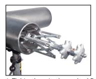
1. Tighten jaws to clamp pipe I.D.
