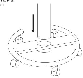
Insert Adjustable Bar (B) into the center of the base.
