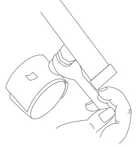
Alternating between locking and non-locking, install three Locking Casters (E) and two Casters (D) into Base (C).
