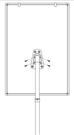
Slide Whiteboard (A) onto the adjustable bar. Secure the whiteboard using four Screws (F).
