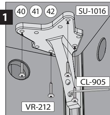
**1** Take off the front support (SU-1016) of the right or the left side depending where you want to place the pedestal by first unscrewing the 4 (VR-212) 25 mm - 1" screw that hold it to the surface **40** **41** or **42** and then the 2 screws of the support (SU-1016) with the key (CL-905). \* If you do not have a side wall, go to step 3.
