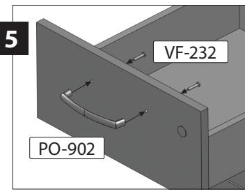
**5** Screw the handles (PO-902) with the screws (VF-232) on the drawers.
