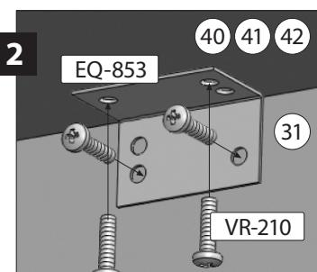
**2** Install the brackets (EQ-853) with the four (VR-210) 16 mm - 5/8" screws between the surface **40** **41** or **42** and the wall besides **31** of where the pedestal will be placed.
