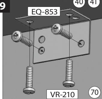
Install the bracket (EQ-853) with the four (VR-210) 5/8" - 16 mm screws between the surface (40) or (41) and the wall (70).
