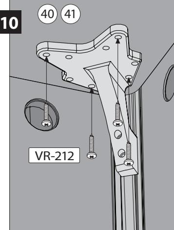
**Attach the surface (40) or (41) to the supports (SU-1016) with the 4 (VR-212) 1" - 25 mm screws using the 4 pre-drilled holes underneath the surface.**
