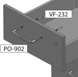
Screw the handles (PO-902) with the screws (VF-232) on the drawers.
