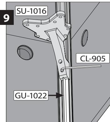
**9** Install the supports (SU-1016) on the legs with the guide (GU-1022) and screw both screws with the key (CL-905).
