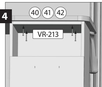
**4** Take off the upper drawer in order to have access to the inside of the pedestal. Install the pedestal to the surface **40** **41** or **42** using the four (VR-213) 32 mm - 1 1/4" screws.
