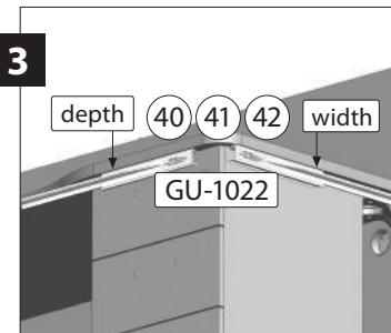
**3** With the guide (GU-1022) which is placed horizontally underneath the surface **40** **41** or **42**, place the pedestal in width and in depth. See below illustration.
