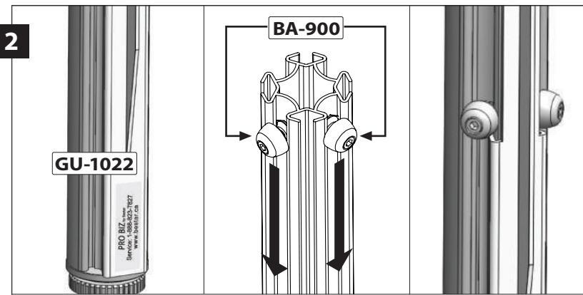
Make sure the adjustable legs (at the bottom) are fully screwed in. Place the guide (GU-1022) on top of the adjustable legs (see picture). Slide the stop bolts (BA-900) into the groove to the guide (GU-1022). Tighten the stop bolts (BA-900).
