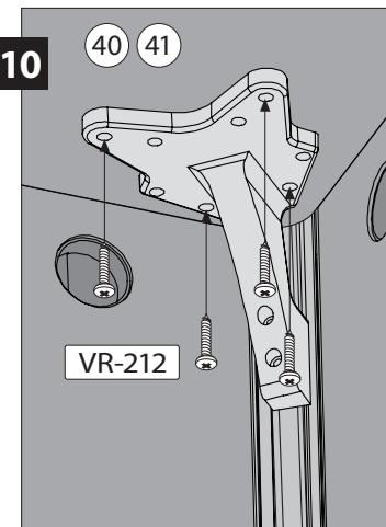
**10** Attach the surface (40) or (41) to the supports (SU-1016) with the 4 (VR-212) 1" - 25 mm screws using the 4 pre-drilled holes underneath the surface.
