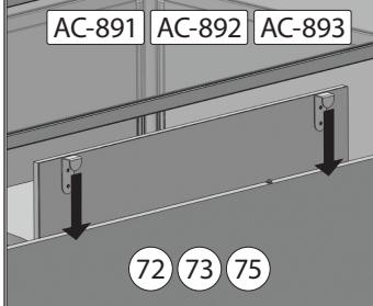
To add a tackboard on the wall (72) (73) or (75), it needs to be installed before sliding the plexiglas AC-891, AC-892 or AC-893.
