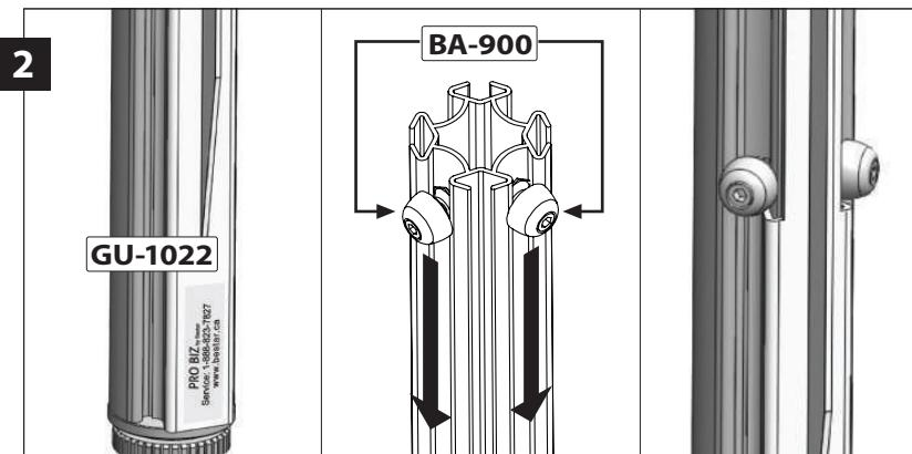
**2** Make sure the adjustable legs (at the bottom) are fully screwed in. Place the guide (GU-1022) on top of the adjustable legs (see picture). Slide the stop bolts (BA-900) into the groove to the guide (GU-1022). Tighten the stop bolts (BA-900).
