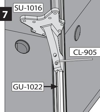
Install the supports (SU-1016) on the legs with the guide (GU-1022) and screw both screws with the key (CL-905).
