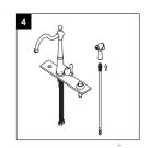
Install the spout through top of sink. From underneath the sink, replace the rubber seal, metal washer and lock nut. Tighten the screws on the lock nut to secure the body.
