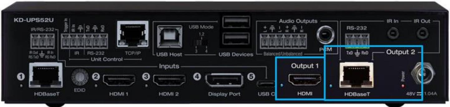
**HDMI (Output 1):** Using an HDMI cable, connect your display or system. For DVI-D/DVI-I sources use an appropriate adapter. For Display Port, use active adapters.
