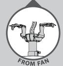
Using the orange wire connectors from the hardware bag, connect the black wire (ungrounded) from the ceiling to the black and the blue wires from the fan. Connect the white wire (grounded) from the ceiling to the white wire from the fan.
