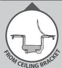
Using an orange wire connector from the hardware bag, connect the 3 grounding wires (green, green/yellow stripe, or bare copper) coming from the ceiling, downrod, and hanging bracket.
