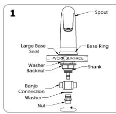
Place backnut onto shank and tighten to underside of worksurface.
