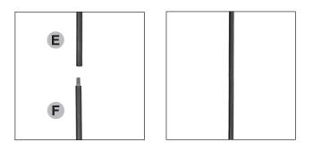
When everything is assembled, insert stake base firmly into the ground. For best results, install on flat ground and ensure that the stake is 90 degrees vertical to the ground.
