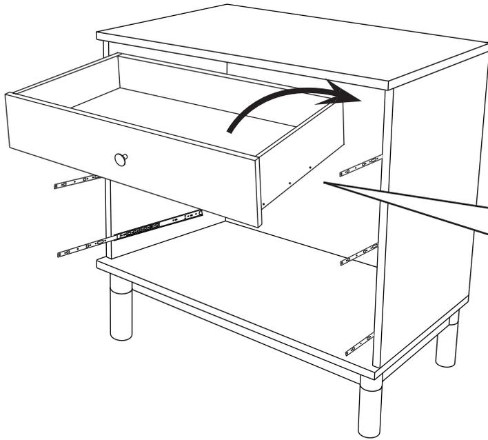
\* Make sure that the drawer is placed on the tabs on the glide rails.
