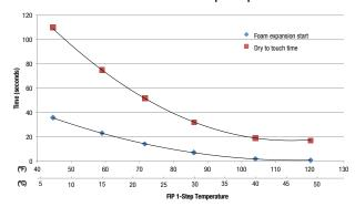
\*Note: Expansion Start Time and Dry to Touch Times are NOT dependent on ambient air temperature. Expansion Start Time and Dry to Touch Times are dependent on FIP 1-Step temperature.
