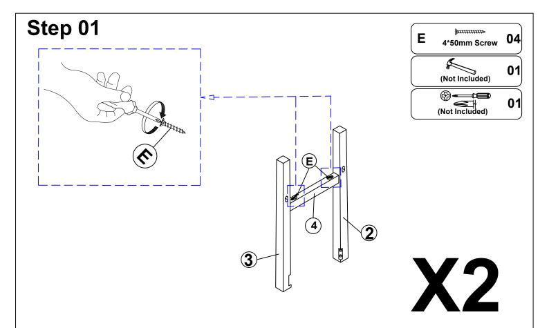
Note: Don't tighten screws until completely assembly!
