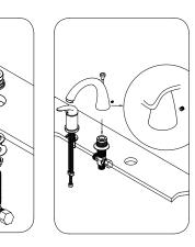
Unscrew the Allen screw in back of the spout. Pull apart the spout from its connector (do not unscrew). Separate the spout flange from the spout. Place o-ring underneath the spout flange and place the flange over the center hole between the handle and hand shower.
