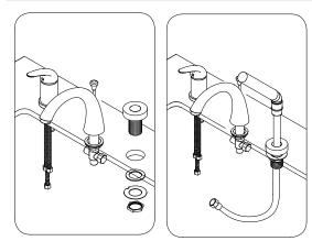
Unscrew the locknut and take off metal and rubber washers.
