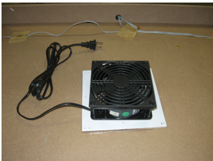
Securely mounted 5 blade axial fan AC120V 50/60 Hz 0.28A 24W 2P
