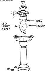
**4.** Fill the fountain with water, ensuring the pump is completely submerged during operation; approximately 1.5 gallons.
