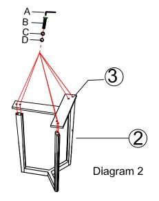
Step 2: Attach mounting bridge (3) on legs (2).
