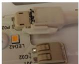
Remove channel cover assembly by applying pressure to sides of channel at opposite ends.
